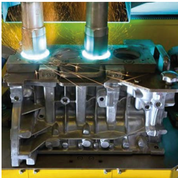
Electric arc wire spraying procedure at BMW
