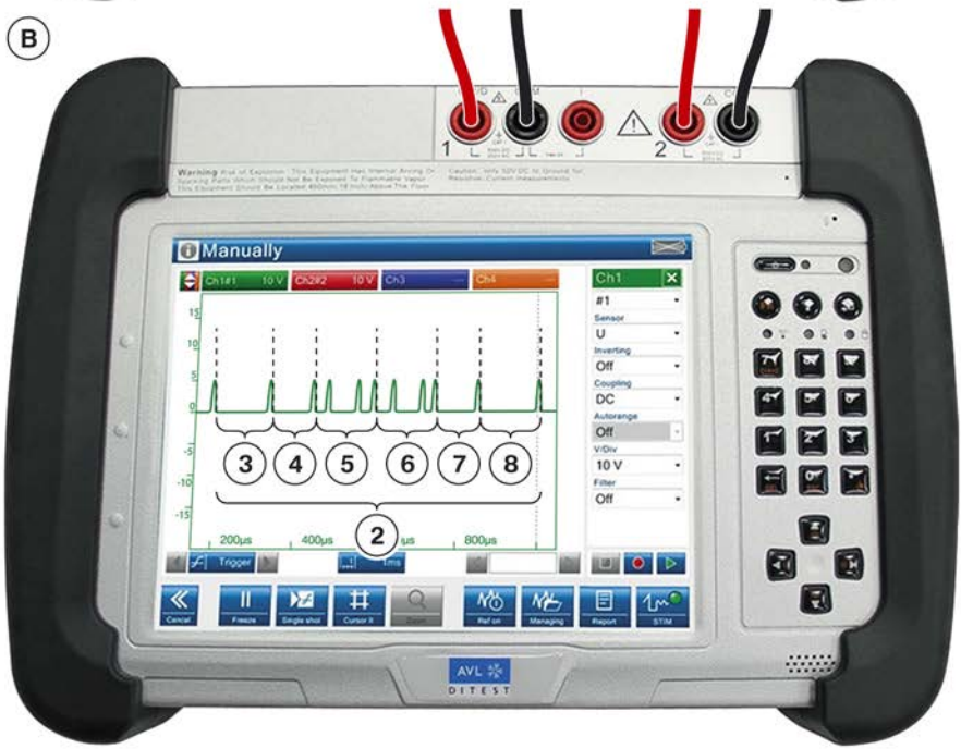
A comparison of air mass signal pulse-width modulation and SENT
