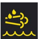
SCR 3, Check Control message in the instrument cluster at warning level 2
