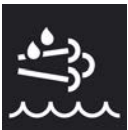
SCR 3, Check Control message in the instrument cluster at warning level 1
