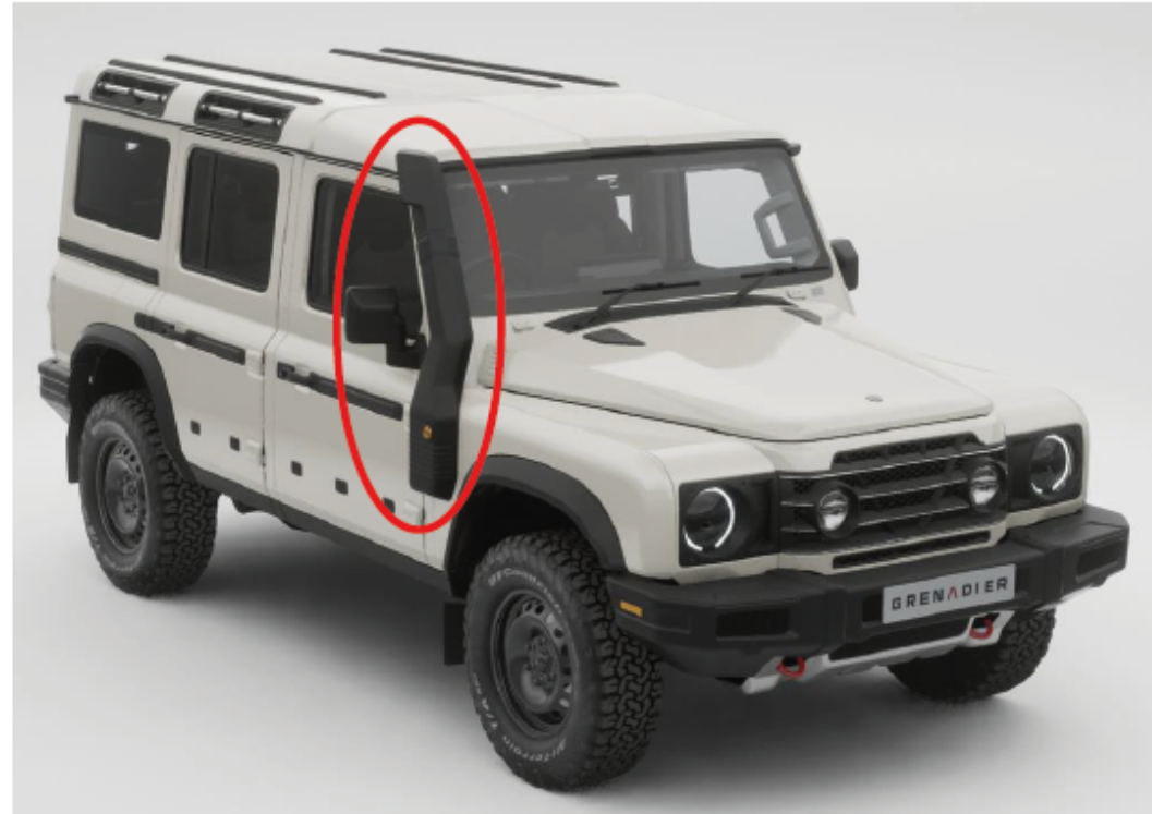
Raised Air Intake mounted to A-Pillar
