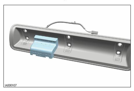
Remove the roof bar wiring harness cover.
