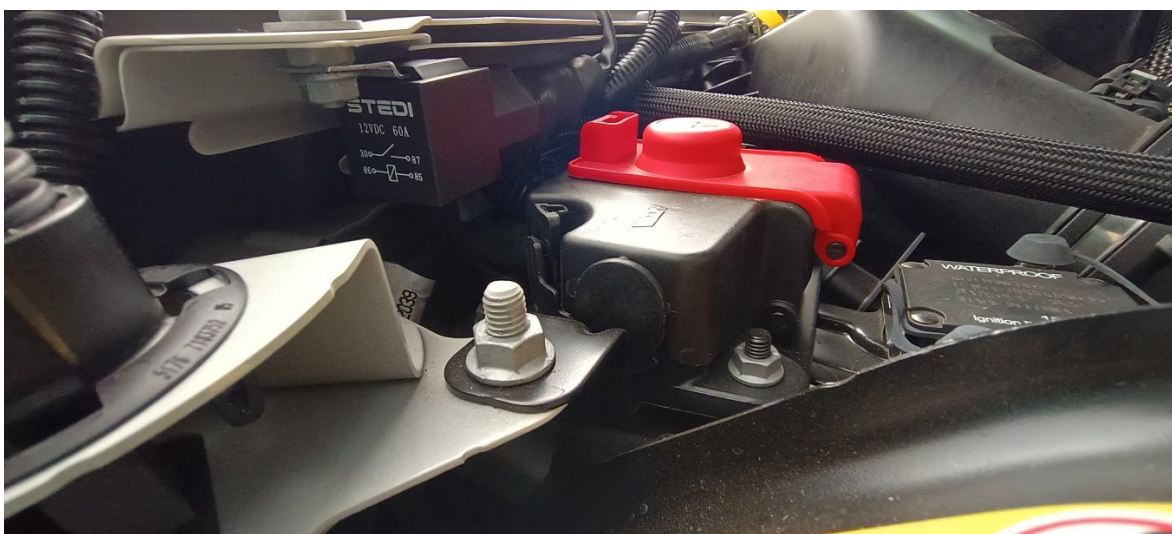
Photo 7: Location and fixing of the relay. The spliced high beam lead from the RHS spot/driving light (in the CSPL tubing) is just visible in the top left corner.
