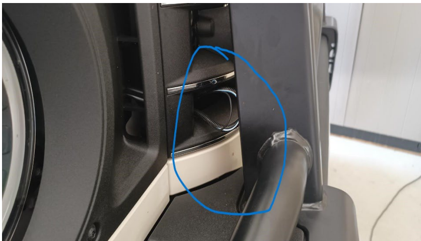
Photo 3: Power leads to the round spot/driving light inboard of the RHS headlight
