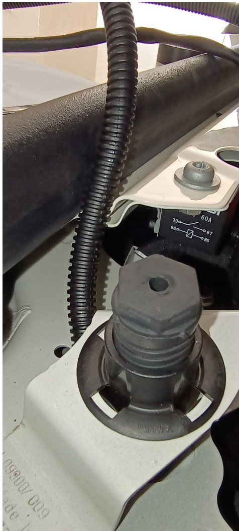
Photo 6: Exit point for spliced high beam lead and location of relay under lip on RHS edge of engine compartment.
