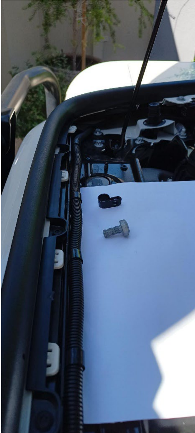
Photo7: Power lead to light bar from relay attached to front rim of engine bay with P clip and 8mm torx bolt
