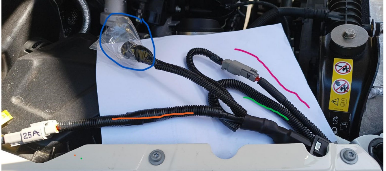
Photo 10: Modified complete wiring loom & connections. Pink is the spliced high beam trigger lead from spot/driving light. Green is the power lead from the relay to the light bar. Orange is the power lead into the relay (far right) from the EXT5 25A outlet and the blue circle is the plastic bag around the small switch from the original wiring loom setup.
