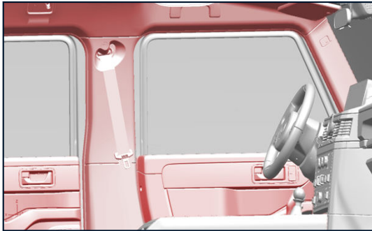
6.16 Required modification free zones for airbags (also counts for passenger side).
