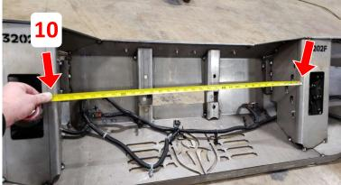
Install Skid Plate Using Factory Bolts. Plug in all Harnesses. Install the Factory Inner Liners to the Bumper. Install all Mesh. If holes need to be re-tapped, use #10-24 Tap.
