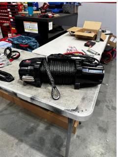
3.) Remove relay pack housing cover from the winch. Then remove the remote plug and plug cover from the housing. You will need to extend the remote plug wire in order to re locate it to mount on the bumper face.
