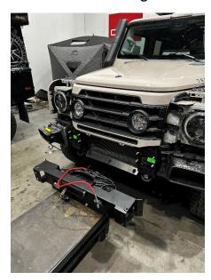
6.) Install bumper/winch assembly onto vehicle. (Some minor trimming of inner grille plastics may be needed to allow winch wiring to clear)
