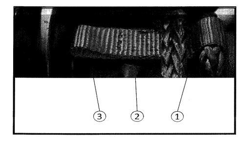
The following image shows the Plasma Lock fully engaged with the Winch Rope inserted **(1)**. You can see the Winch Rope wrapped around the Winch Drum and Plasma Lock four times **(2)** with the
