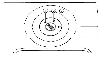
Apply pressure to the foot brake, turn the key to position (3) until engine starts. Once the engine has started, release the key. This will allow the key to rotate back to position (2).
