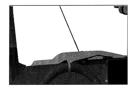
If you see either of the above, then the Winch Rope has reached its maximum extension length. The friction effect between the Winch Rope and Winch Drum will start to fail, if the Winch Rope is spooled out any further.
