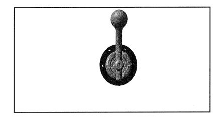
Check that the Freespool Lever is in a vertical position, secured against the lowest part of the cam extrusion.
